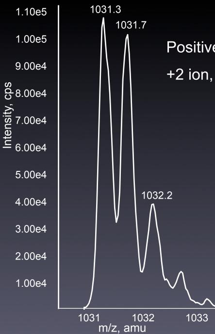
Positive Enhanced Resolution Scan +2 ion, MW= 2060.6
